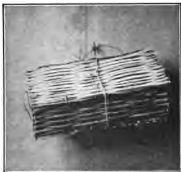
FIG. 204.—An example of French economy. An 11-pound cut flower basket for parcel post shipment made of split cane and requiring but a fraction of the material necessary for a box made of sawed boards. (U. S. Consular Bureau.)
